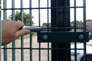
**Finding:** There is/are finger entrapments in the panels and the item fails to meet the requirements of BS EN 15312
